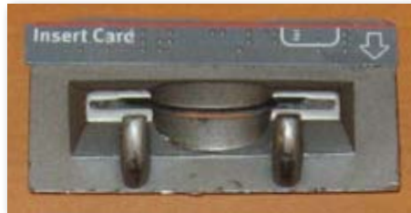
Skimming Device Installed Over Card Slot
